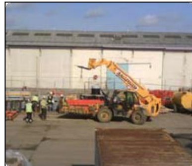
Attachment and load incorrectly positioned
