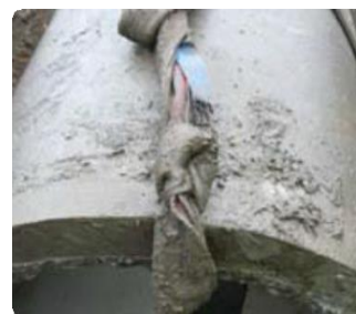
Fibre slings with knots
