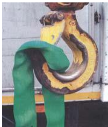
Conventional Safety Hook with Continuous Webbing Sling
